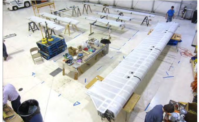
One thousand square feet of fabric was needed to resurface all of the control surfaces.
