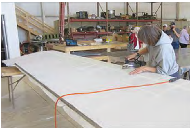
After the fabric was glued and riveted to the aluminum frame, heat was applied to shrink the fabric. This gave it a smooth, tight surface.
